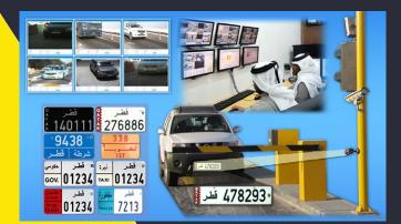
ANPR is a technology that provides automated access on number plate contents, extracting numbers and alphabets within a fraction of a second, and converts it to a computer recognizable format.
